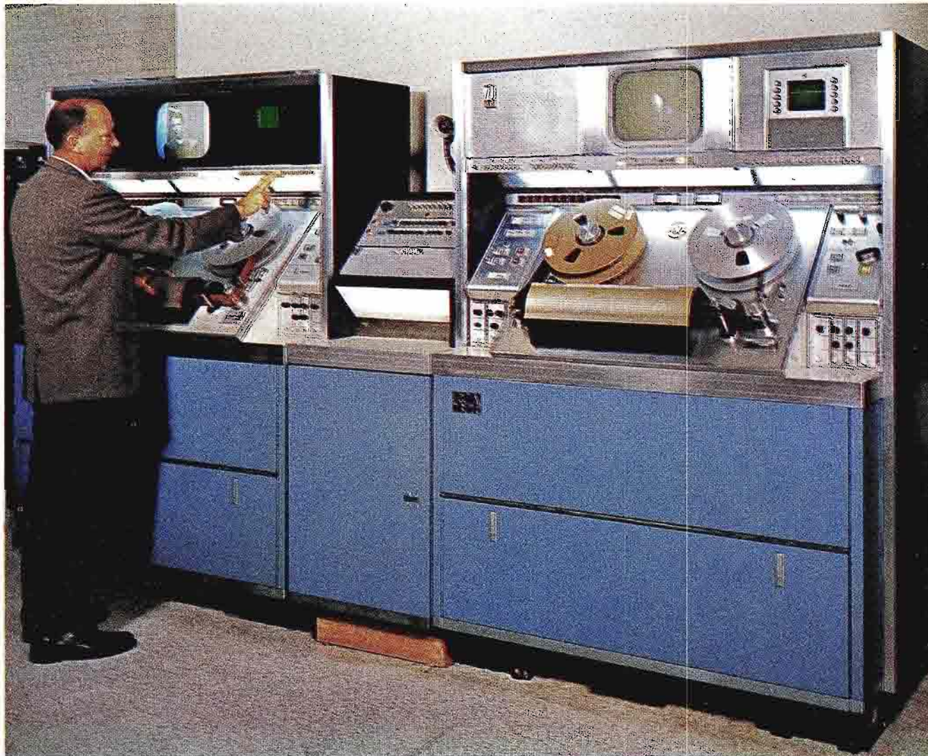
HIGH BAND COLOR TAPE production facility is provided by TR-70 recorder (right). WSJS was the first TV station to install this highband model. Also shown is TR-22 recorder, which has since been highband retrofitted, and custom intercom and input and test signal selection panels (center).
